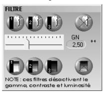
The configuration made in this way by the user will be applied to the panoramic image coming from the I-MAX TOUCH 3D by left-clicking on the icon with the mouse. By clicking a second time the filter is removed. NB: when the configurable filter is used, the gamma, contrast and brightness sliders will not function.
